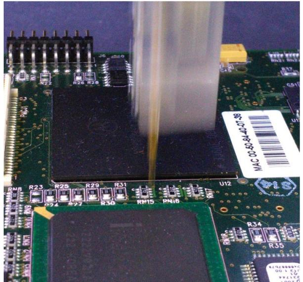
*The mobile probe type "Flying probe" in action, the image of the flowing head is blurred due to the high speed of the probe movement*
