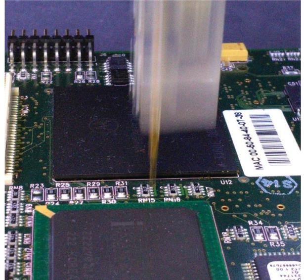
*The mobile probe type "Flying probe" in action, the image of the flowing head is blurred due to the high speed of the probe movement*
