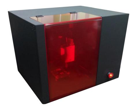
Automatic system for detecting counterfeit, relabeled or defective electronic components in BGA packages
