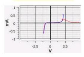
Detection of the defective output of the investigated microcircuit in the BGA package. The figure shows the difference in signatures for the output of the investigated chip and the original chip. Defect is marked in red
