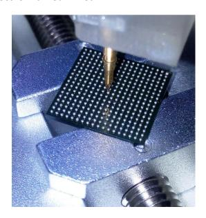
Determination of the pinout location of the BGA chip under investigation by the fully automatic optical scanner integrated into EyePoint B10
